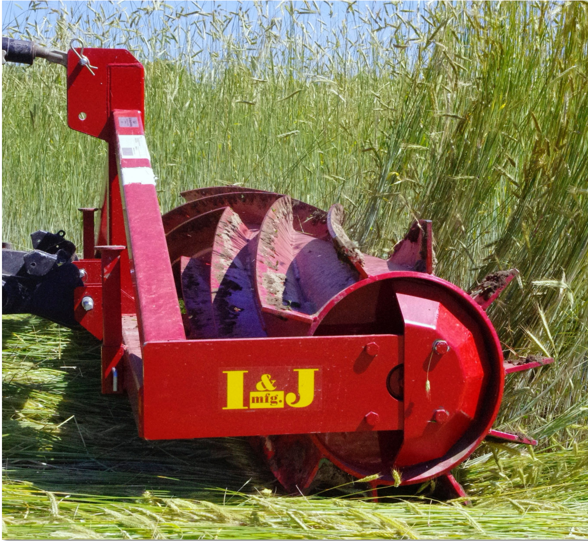
I & J Roller-Crimper (10 ft wide cylinder, 2625 lbs. water-filled weight)
